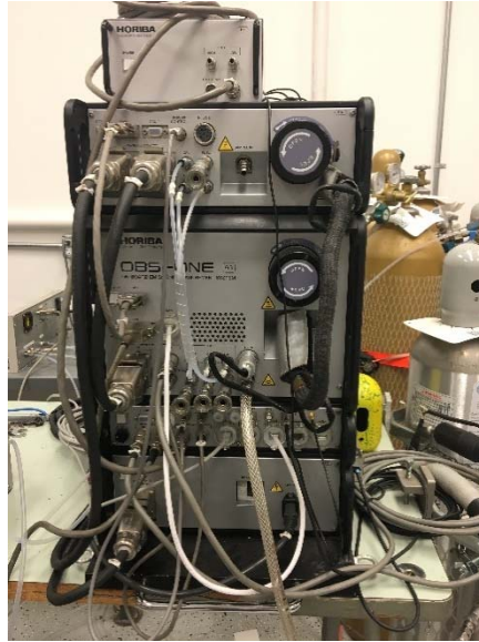
Figure 20: Horiba® OBS-ONE Portable Emissions Measurement System
