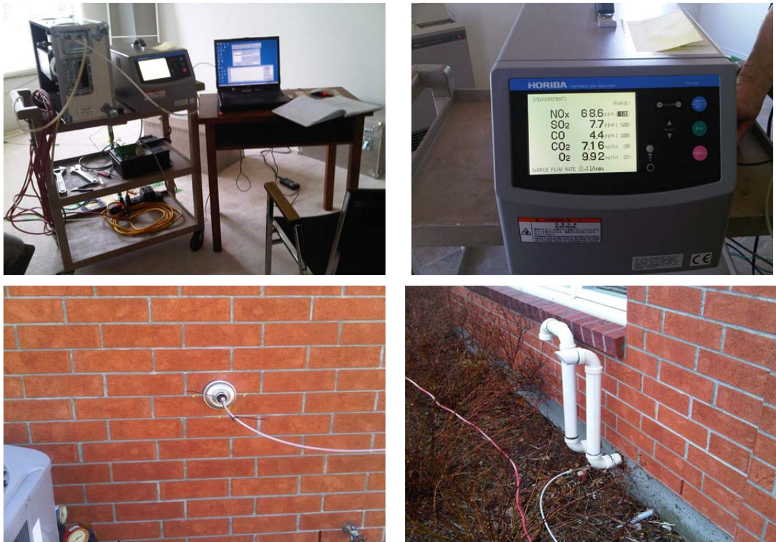
Figure 17: Flue Gas Emissions Measurement Set-up and the Sampling Lines of the DV Wall and Condensing Furnaces Installed in the Experimental and Control Houses
