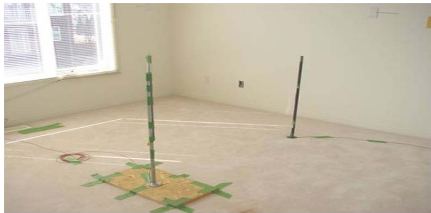
Figure 3: Photographs of Bedroom 2 Location of Thermocouples on Metal Pipe Stands
