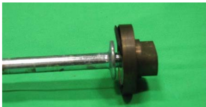
Figure C-30 - PRV 211 Gasket (Still Assembled), Side View
