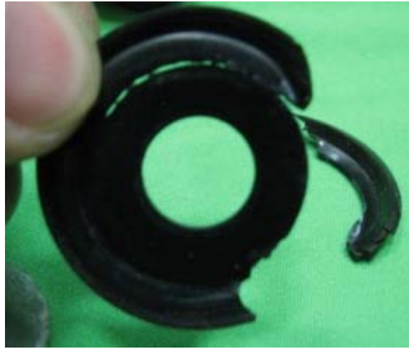
Figure C-31 – Cracked Gasket from PRV 211
