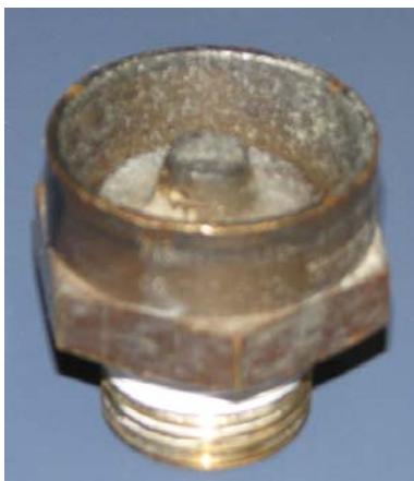
Figure C-9 – Paint Speckles on PRV 19
