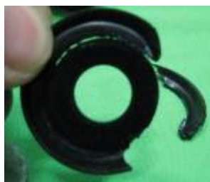
Figure 46. PRV 211 — perforated seat disc.
