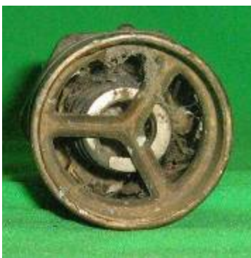
Figure C-1. PRV 80 — debris inside valve.
