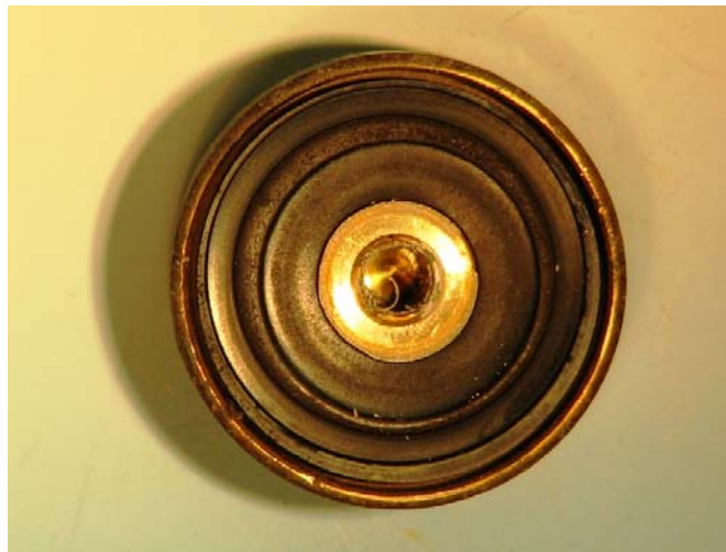
Figure C-5 - PRV 7 Gasket (Overhead View)
