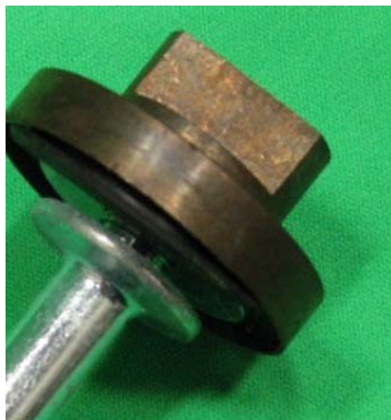
Figure C-29 – PRV 211 Gasket (Still Assembled)
