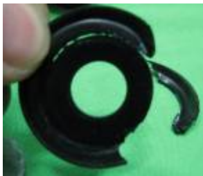
Figure C-2. PRV 211 — perforated seat disc.
