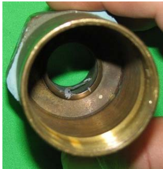
Figure C-16 - PRV 75 with Thread Sealant After Gasket was Removed
