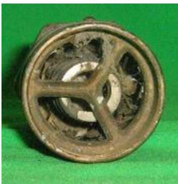
Figure 45. PRV 80 — debris inside valve.
