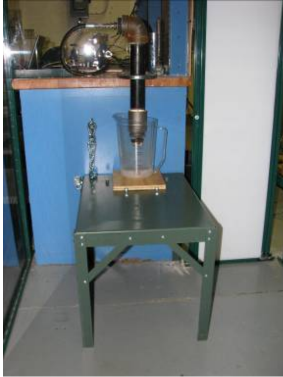
Figure 18. PRV test stand — view of PRV.
