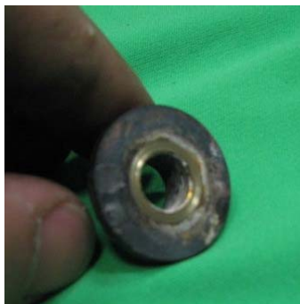
Figure C-27 – PRV 211 Corrosion of Bottom Flange
