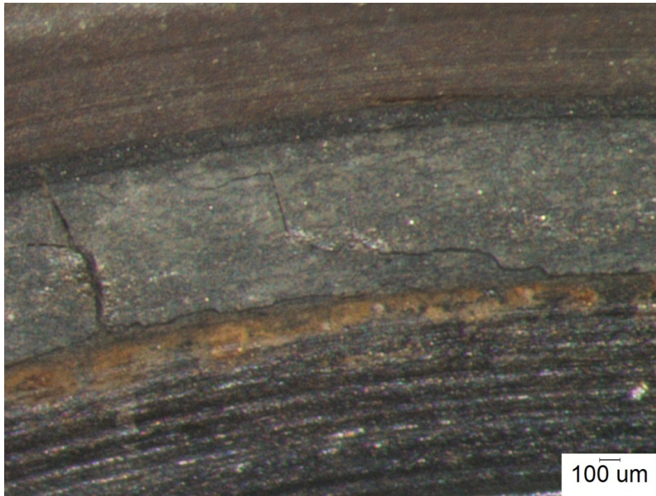
Figure 15 – Higher Magnification View of Radial and Circumferential Cracks in the Surface of the Outer Circumferential Ring in PRV 270
