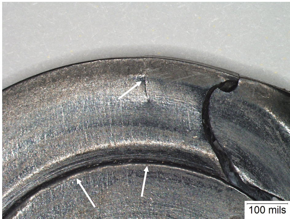
Figure 12 - Circumferential and Radial Cracks in the Gasket from PRV 211
