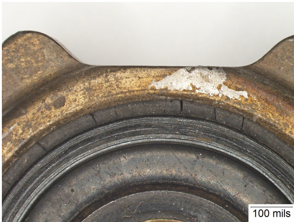
Figure 16 - Radial Cracks in the Outer Circumferential Ring on the Sealing surface of the Gasket from PRV 329 The gasket is still in the holder
