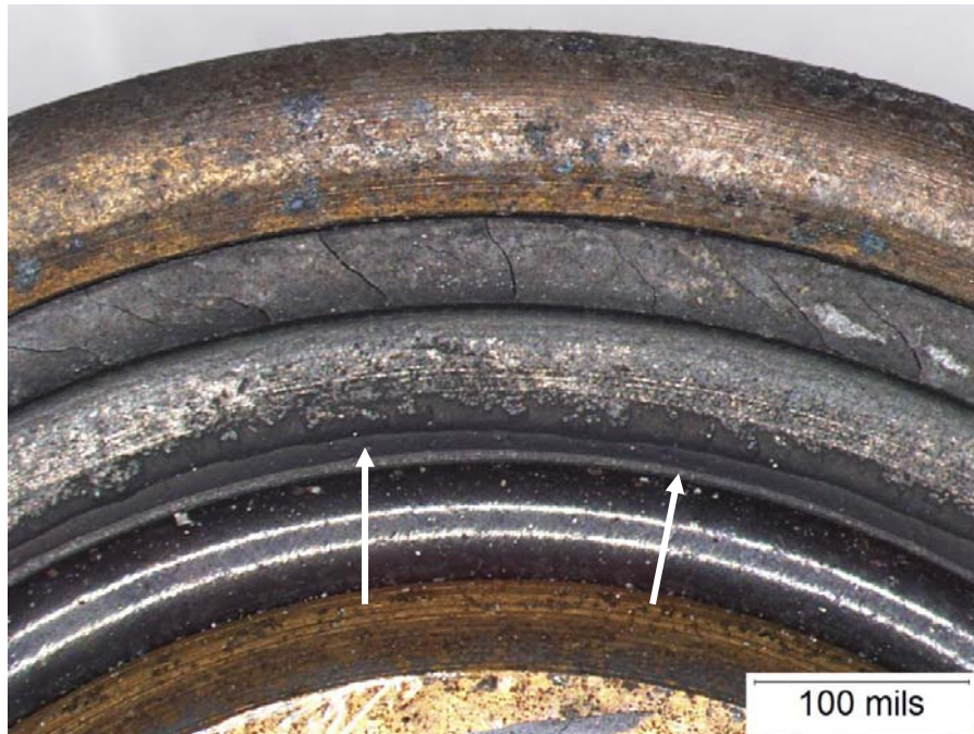
Figure A-43. Material Pulled Out of the Surface of the Sealing Region (Arrows) and Cracks in the Outer Circumferential Ring of the Gasket from PRV 250
