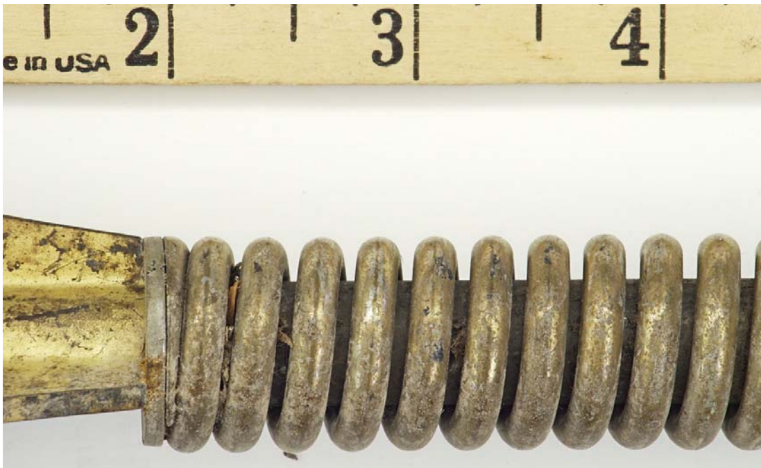
Figure A-28. White Residue on the Spring Coil Surfaces and Debris Inside the Spring
