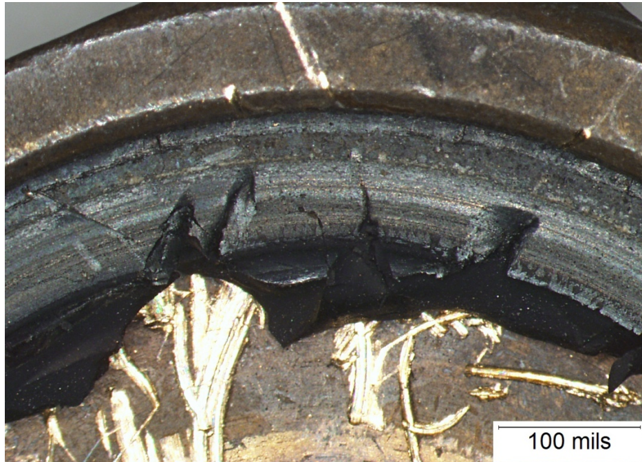
Figure A-9. Portion of the Gasket Stuck in the Seat Holder from PRV 173. This gasket contained radial cracks in the outer circumferential ring and it broke into many small pieces when it was pulled to remove it from the holder
