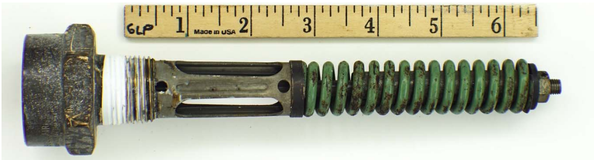
Figure A-10. PRV 274 Did Not Open when Tested during the Initial Study but Opened at 328 psig when Retested During the Present Study
