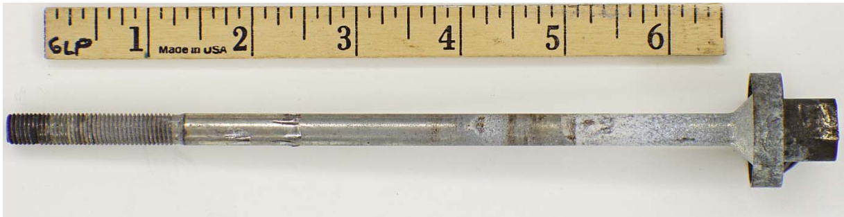
Figure A-46. White Corrosion Products, Rust, and an Interaction Band on the Surface of the Valve Stem from PRV 398
