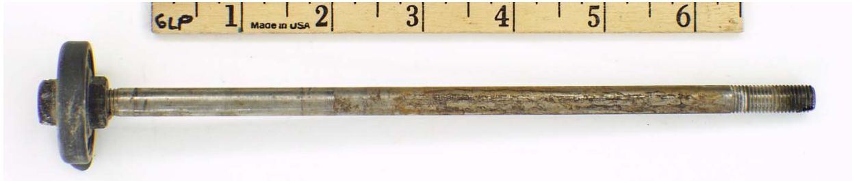
Figure A-31. Corrosion on the Surface of the Valve Stem from PRV 102
