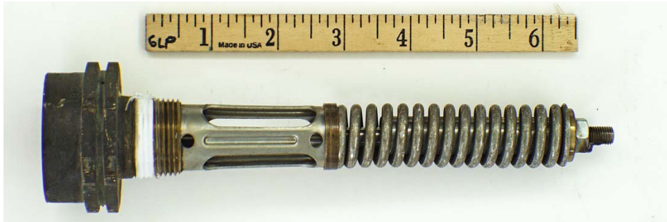
Figure 28 - Absence of Rain Cap Line on the External Surface of the Body of PRV 120
