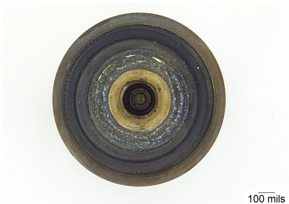
Figure 17 - Sealing Surface of the Gasket from PRV 343 Note the roughened surface in the outer circumferential ring and the compression set rings are somewhat off center; the latter condition perhaps indicating misalignment.
