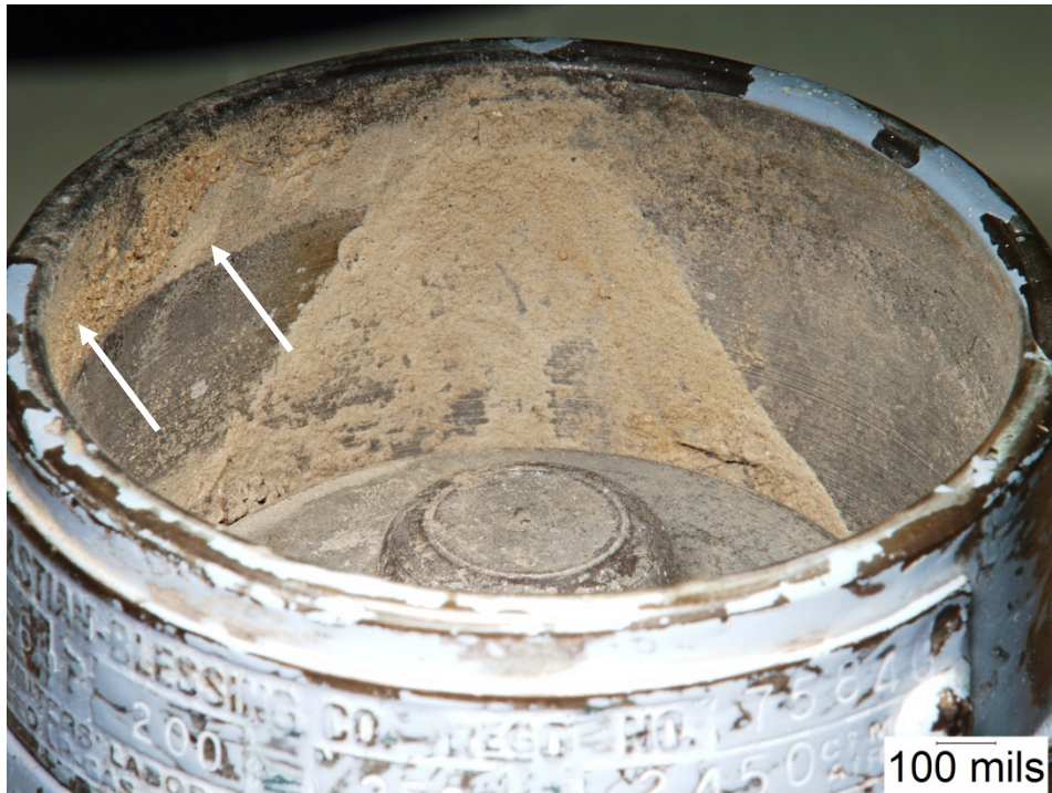
Figure A-29. Blue Paint on the External Surface and Dried Mud on the Internal Surface of PRV 102. A faint internal rain cap line was present (arrows)
