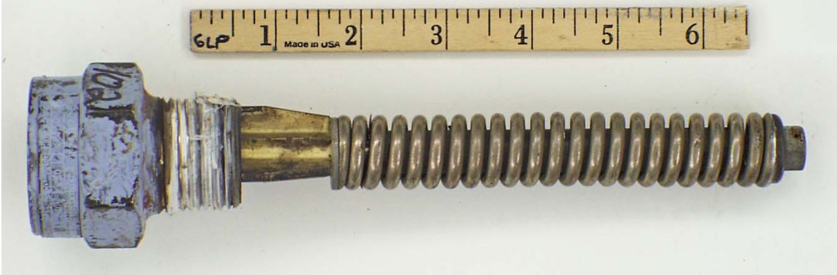
Figure A-27. Appearance of PRV 102. Note the absence of corrosion or discoloration of the components.
