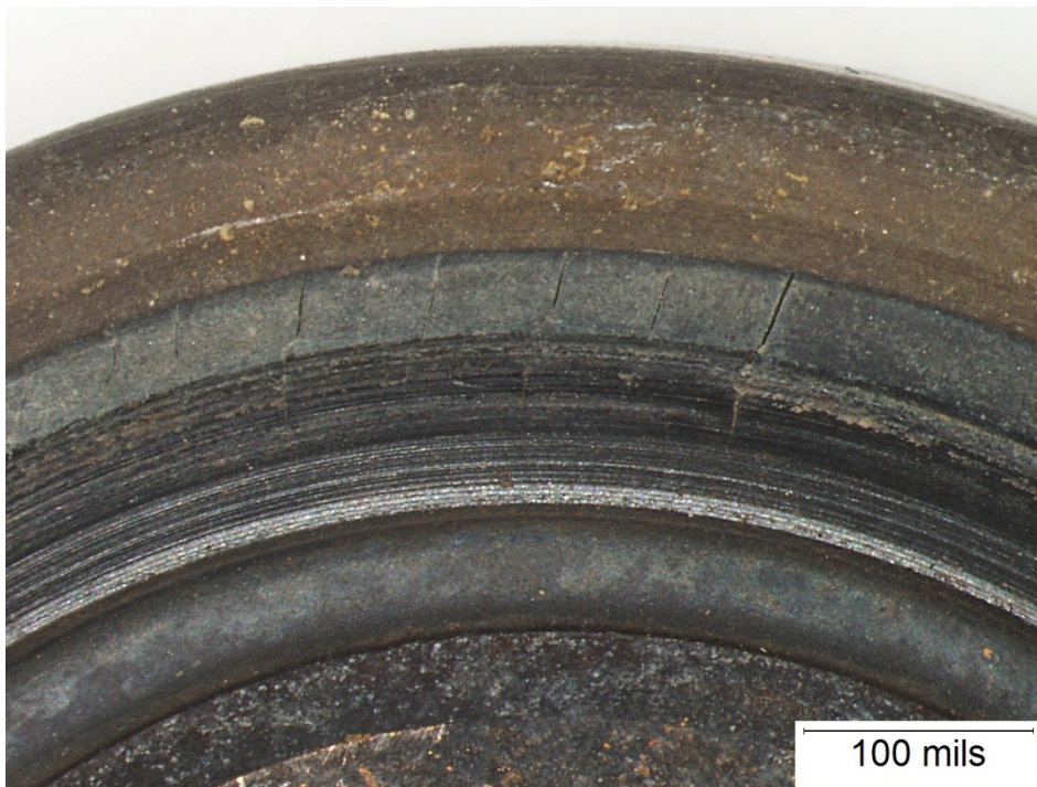
Figure 14 - Radial cracks in the Outer Circumferential Ring (Beyond the Seal Ring Surface) in the Gasket from PRV 270
