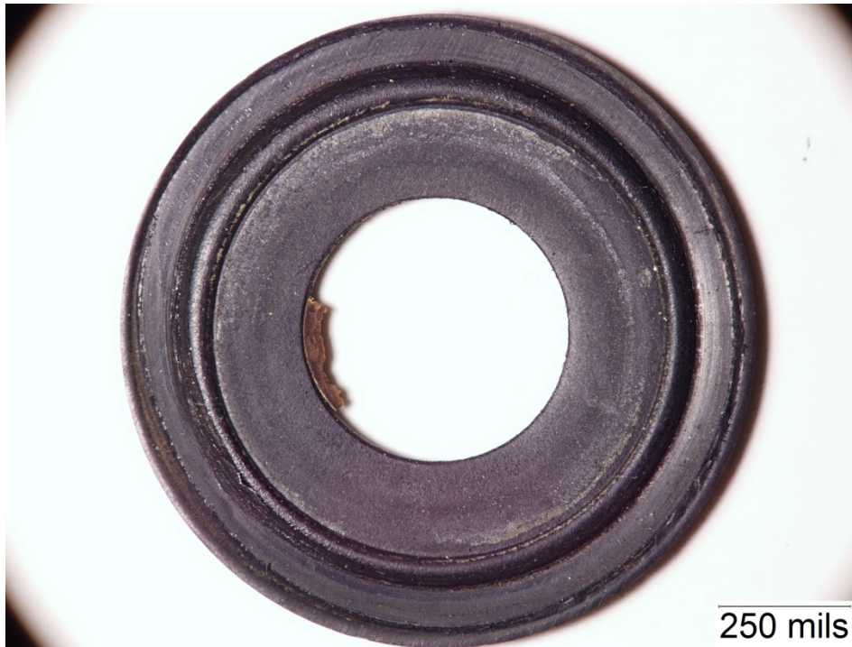
Figure A-24. Sealing Surface of the Gasket from PRV 350 Showing That the Compression Set Lines Were Somewhat Off Center Indicating Possible Alignment Problems
