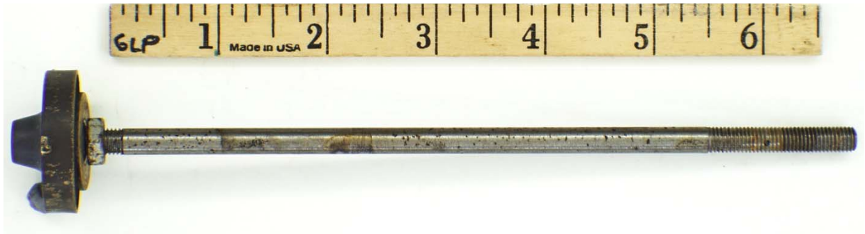
Figure A-22. Corrosion on the Surface of the Valve Stem from PRV 350
