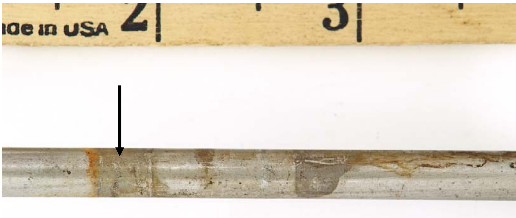
Figure A-19. Corrosion/Interaction Line on the Valve Stem at the Location of the Guide Washer (Arrow) and Additional Corrosion on the Valve Stem Below That Region
