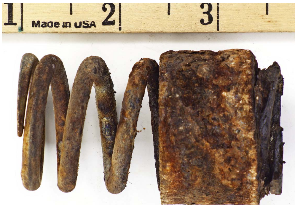
Figure A-4. Corroded Spring and Sleeve Surrounding the Spring from PRV 62
