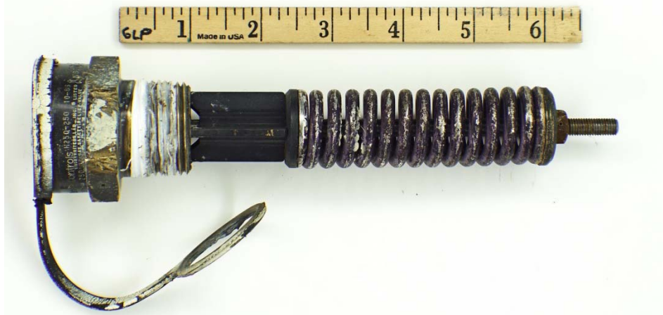
Figure 31 - Internal Rain Cap/Plug on PRV 350
