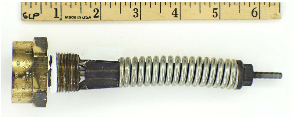
Figure A-44. PRV 5. Note the Absence of a Washer between the Guide Spacer and the Spring and the Bow in the Spring.
