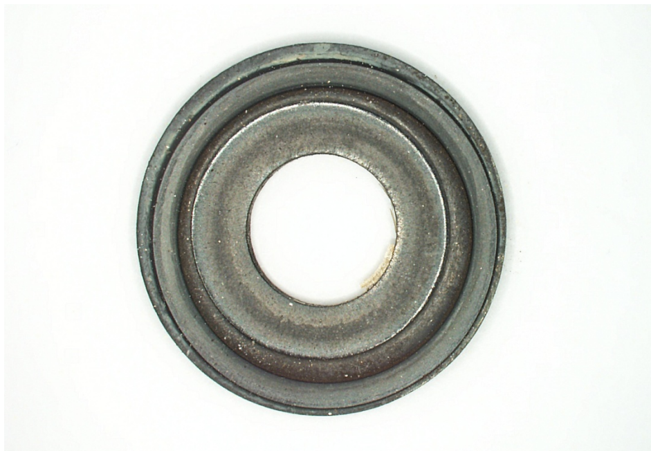
Figure 9 - Compression Set Rings on the Active/Sealing Surface of the Gasket From PRV 7 Note that the compression set rings are somewhat off center.
