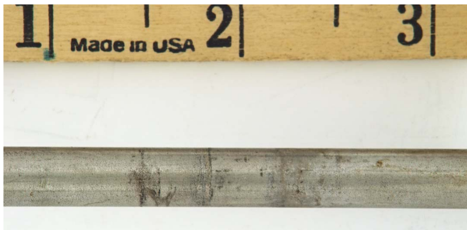
Figure A-33. Corrosion/Interaction Marks on the Surface of the Valve Stem from PRV 102. This region was 180 degrees from the area shown in Figure A-30.
