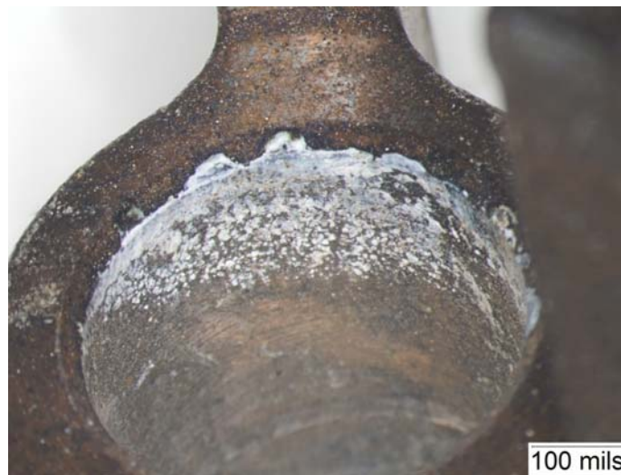
Figure A-48. White Corrosion Products on the Inner Surface of the Guide Spacer and General Oxidation of the Guide Spacer Surfaces from PRV 398
