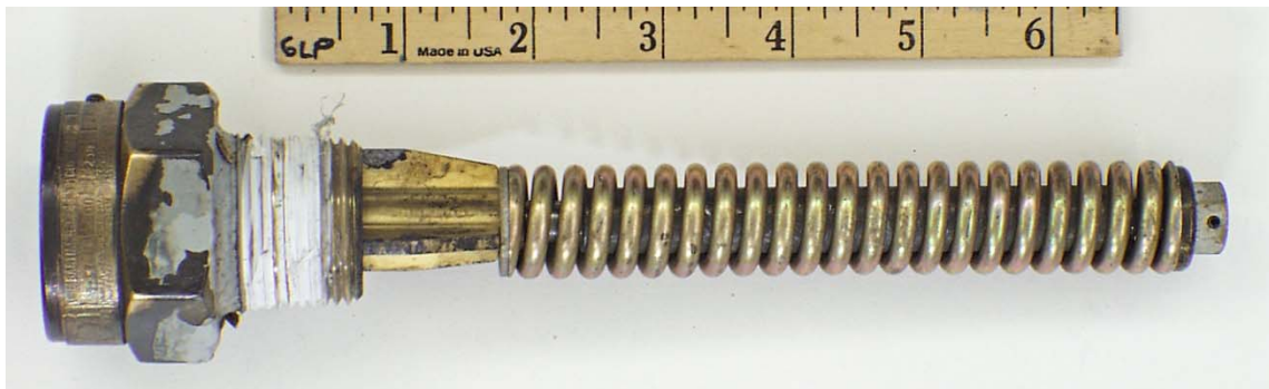
Figure A-40. PRV 250, Did Not Open During Initial Performance Testing Program
