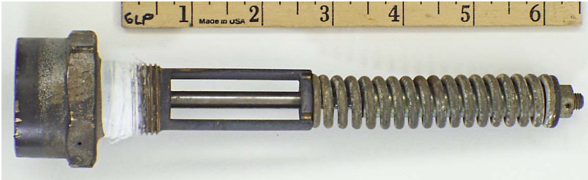
Figure A-53. Appearance of PRV 343
