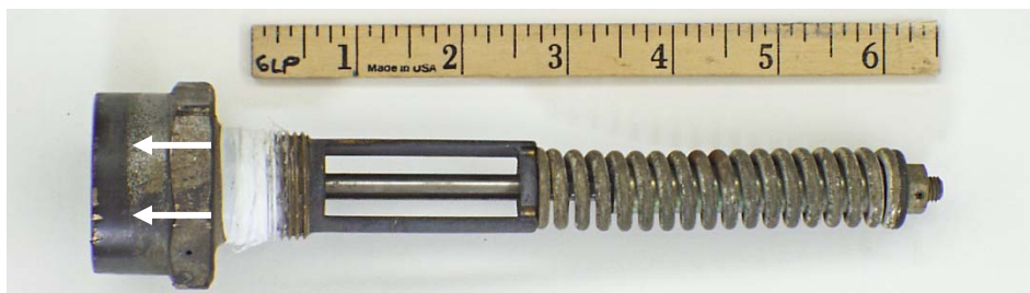
Figure 27 - Discolored External Surface of Valve Body under Rain Cap Line on PRV 343
