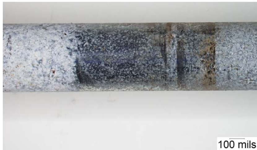
Figure A-47. Higher Magnification View of the Corrosion Products and Interaction Band on the Surface of the Valve Stem from PRV 398
