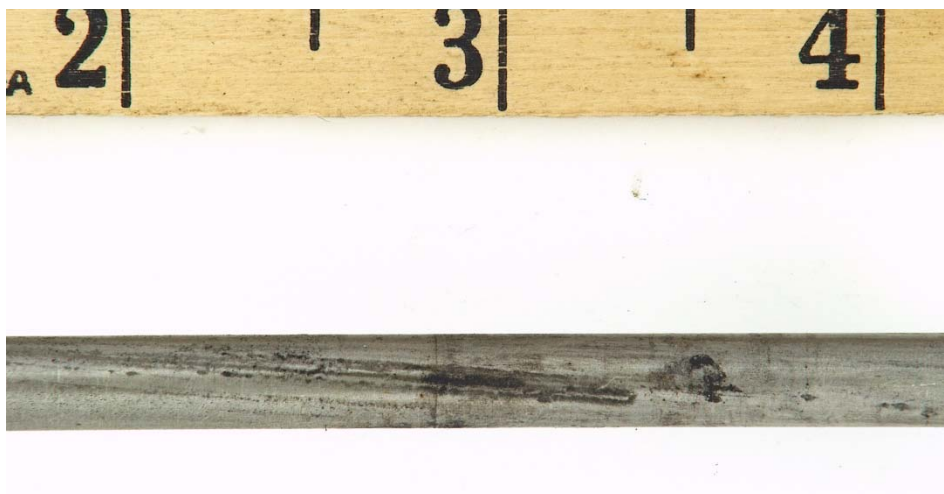
Figure A-14. Region of Interaction between the Valve Stem and the Guide Washer 180 Degrees from the Region Shown in Figure A-13, PRV 274
