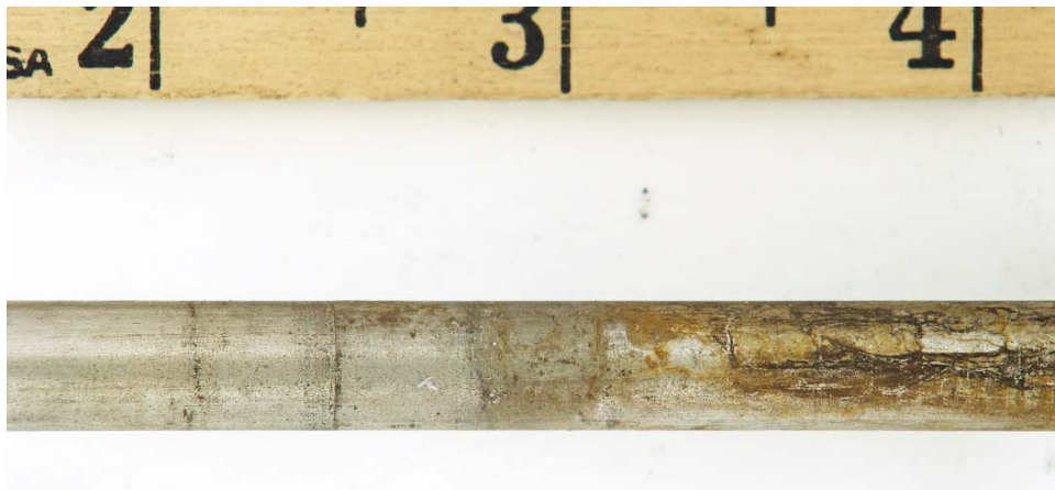
Figure A-32. Higher Magnification View of the Corrosion and Interaction Region on the Valve Stem from PRV 102. The interaction region is where the valve stem contacts the inner surface of the guide spacer.
