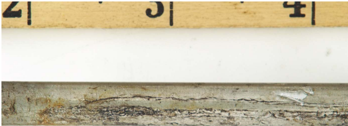
Figure A-34. Higher Magnification View of Another Region of corrosion on the surface of the Valve Stem from PRV 102
