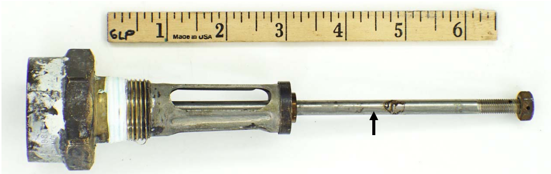
Figure A-6. PRV 173 after the Spring had been Removed Showing Discoloration of the Spacer and Corrosion on the Valve Stem (Arrow)
