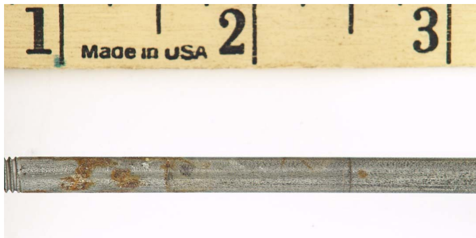
Figure A-59. Higher Magnification View of the Corrosion and an Interaction Line on the Surface of the Valve Stem from PRV 19
