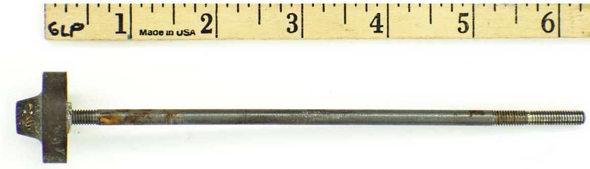
Figure A-58. Corrosion on the Surface of the Valve Stem from PRV 19
