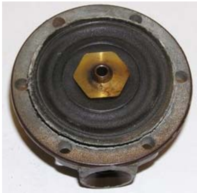
Figure 11: First-Stage Outlet (Regulator #13)
