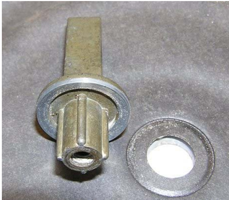
Figure 7: PRD Stem and Seal with Diaphragm
