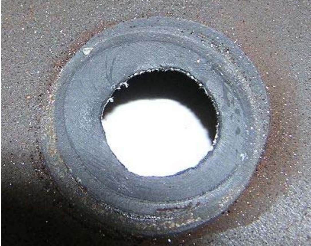
Figure 4: Debris on Seal Between Diaphragm Bottom and Control Linkage
