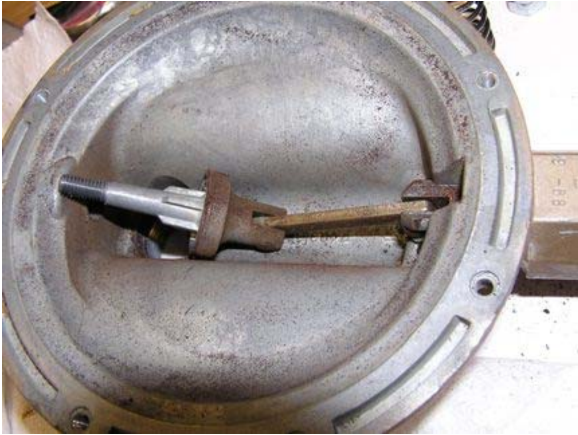
Figure 3: Bottom Half of Body (Regulator #72)
