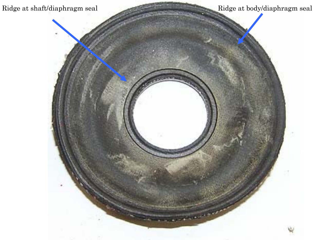
Figure 3: Main Diaphragm of #538. Note the Zig-Zag marks on the surface were put there during disassembly of the diaphragm/shaft.
