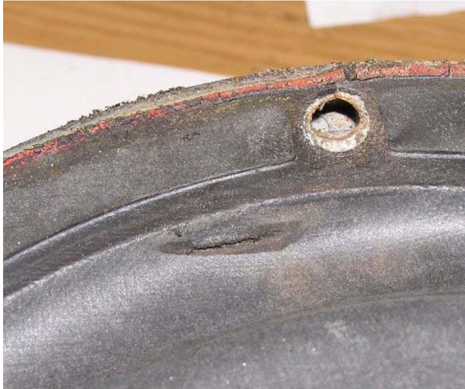
Figure 5: Cut on Bottom of Regulator #361 Diaphragm
