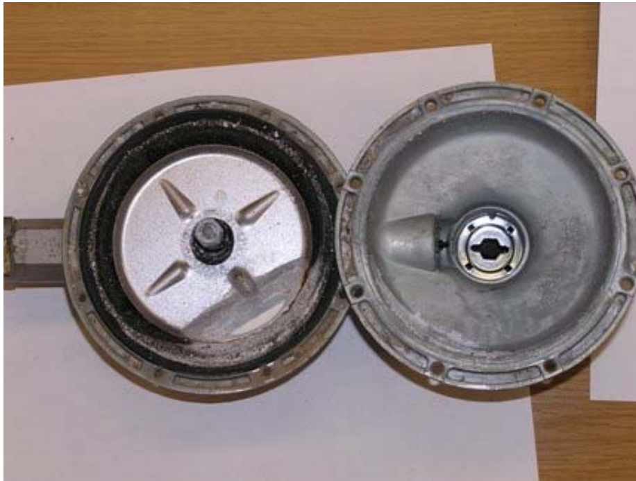
Figure 2: Inside of Regulator #353 Body
