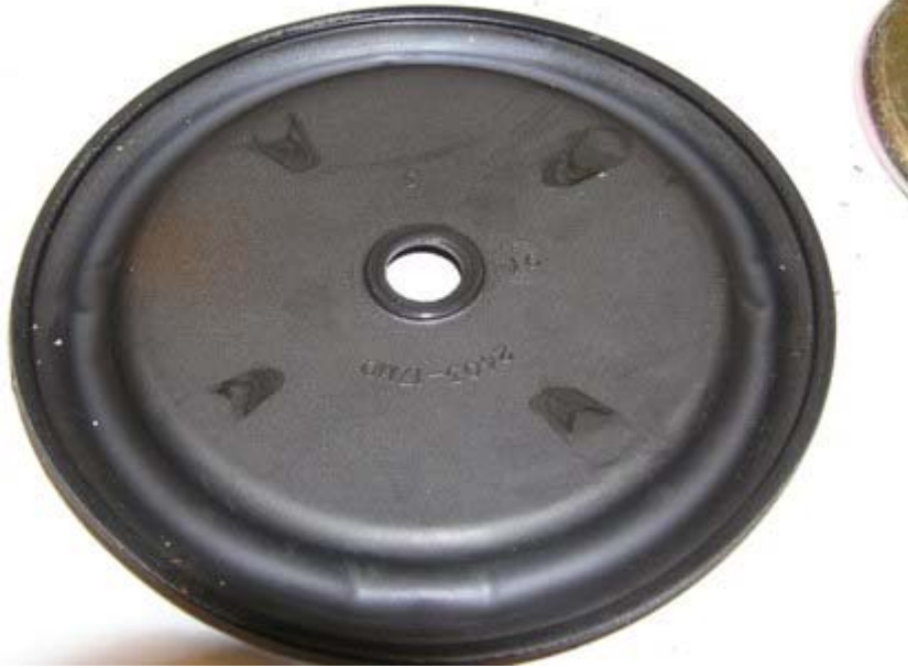
Figure 6: Bottom of Second-Stage Diaphragm (Regulator #13)
