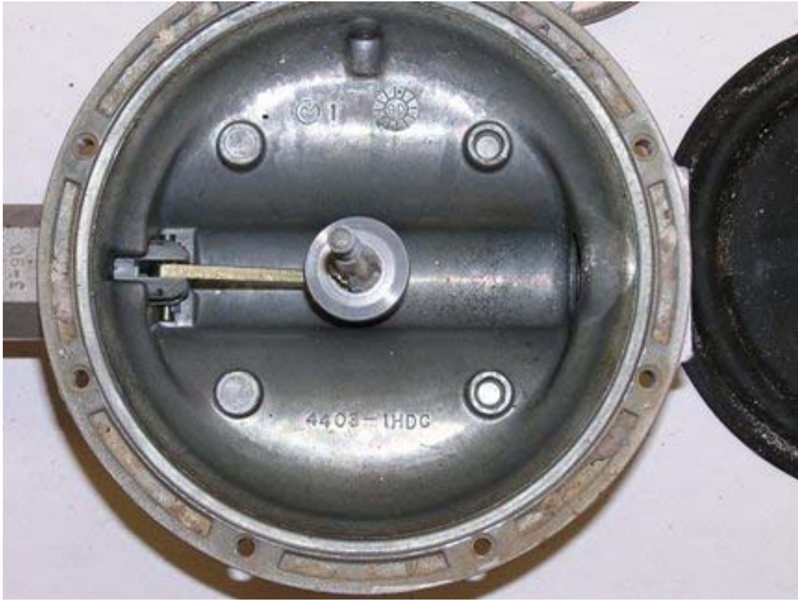
Figure 5: Bottom Half of Body (Regulator #353)
