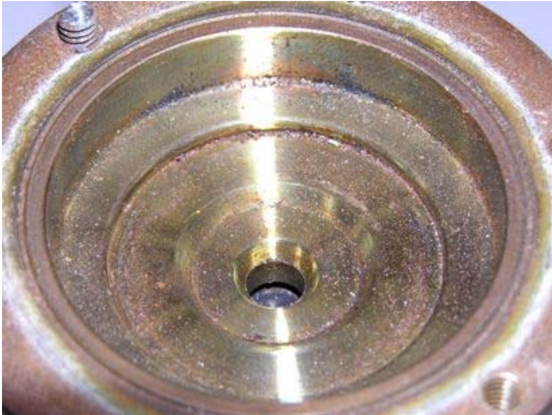
Figure 9: Inlet to the Second-Stage (Outlet of the First-Stage) (Regulator #13)
