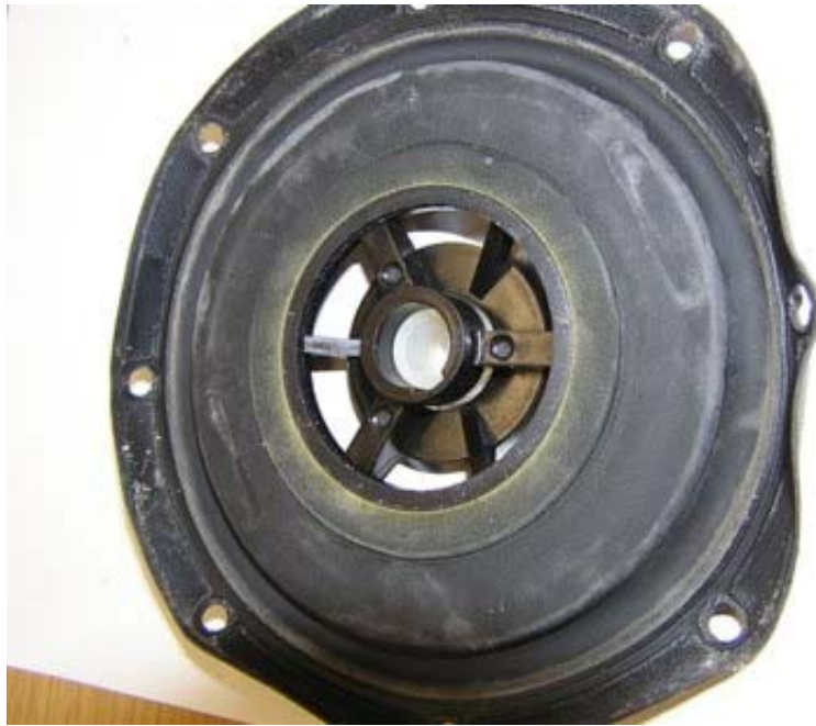
Figure 4: Bottom of Second-Stage Diaphragm (Regulator #490)
