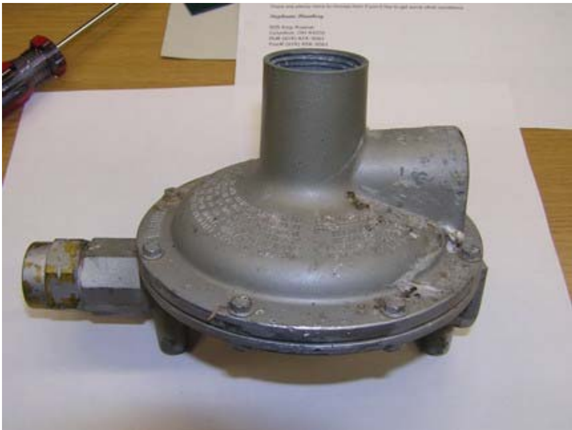
Figure 1: Regulator #353 (Cap Removed)
