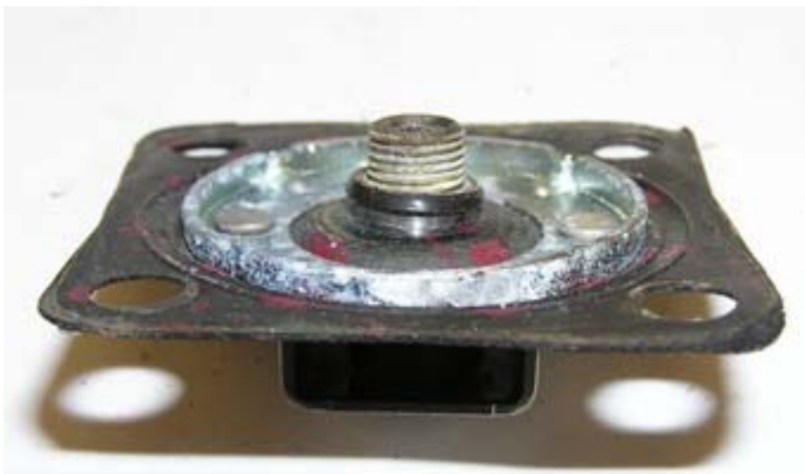
Figure 9: First-Stage Diphragm (Regulator #490)
