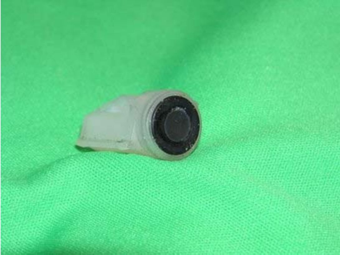
Figure 6: Seat Disc from Control Linkage (Regulator #571)
