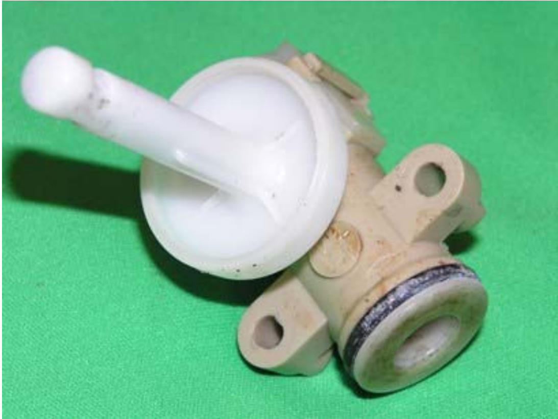
Figure 5: Control Linkage Assembly (Regulator #571)
