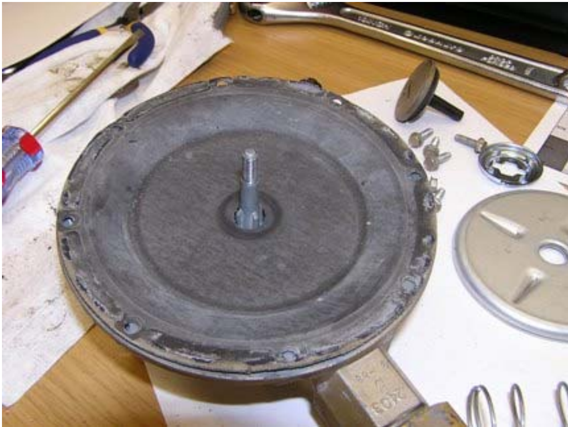
Figure 2: Top of Diaphragm (Regulator #72)
