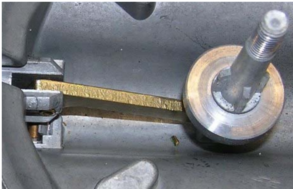
Figure 8: Close-up of Debris in Bottom Body of Second-Stage (Regulator #13)
