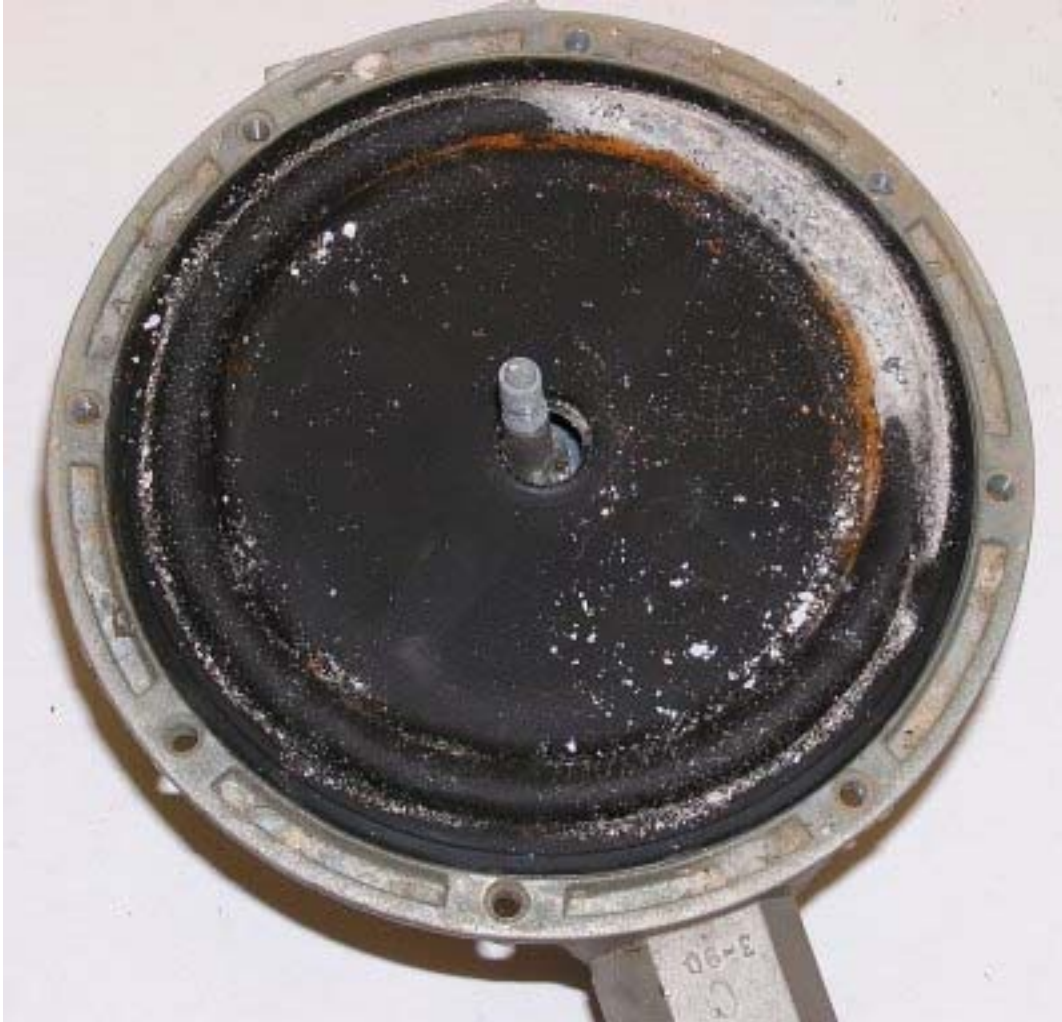
Figure 4: Debris on Diaphragm and PRD Stem (Regulator #353)
