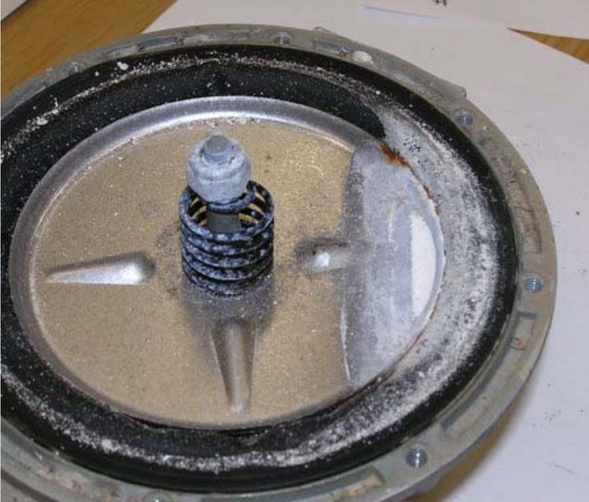
Figure 3: Corrosion and Residue on Plate (Regulator #353)
