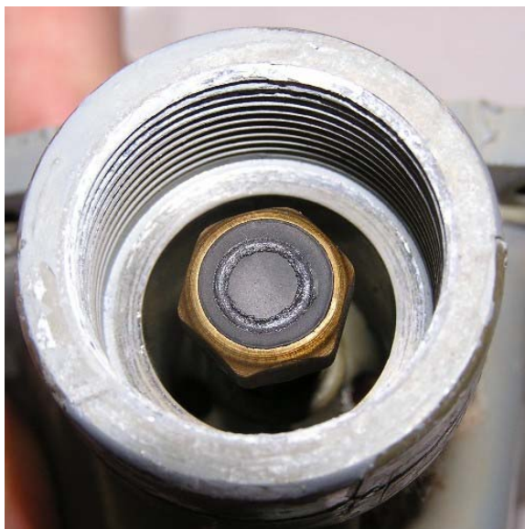
Figure 78. Regulator 383 — seat disc.
