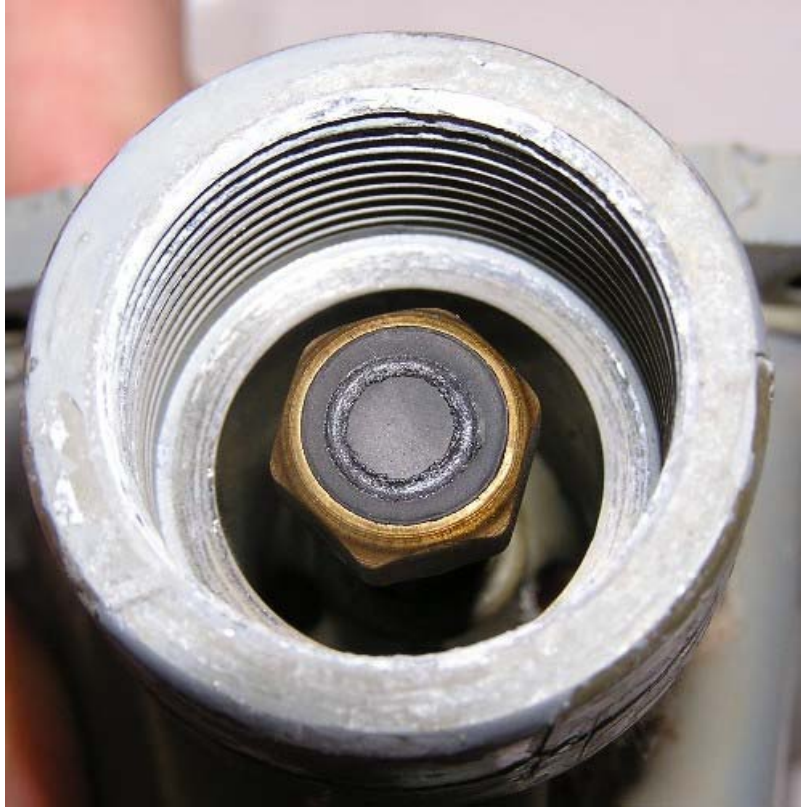
Figure 6: Inlet Seat Disc on Regulator #383
