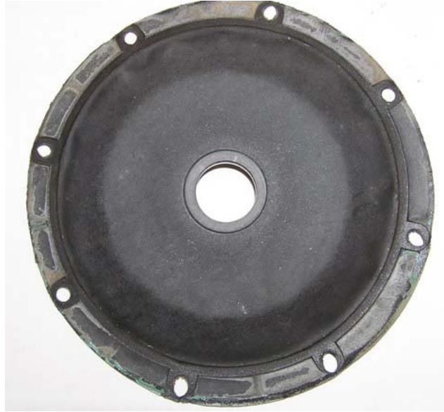
Figure 5: Underside of Regulator #42 Diaphragm
