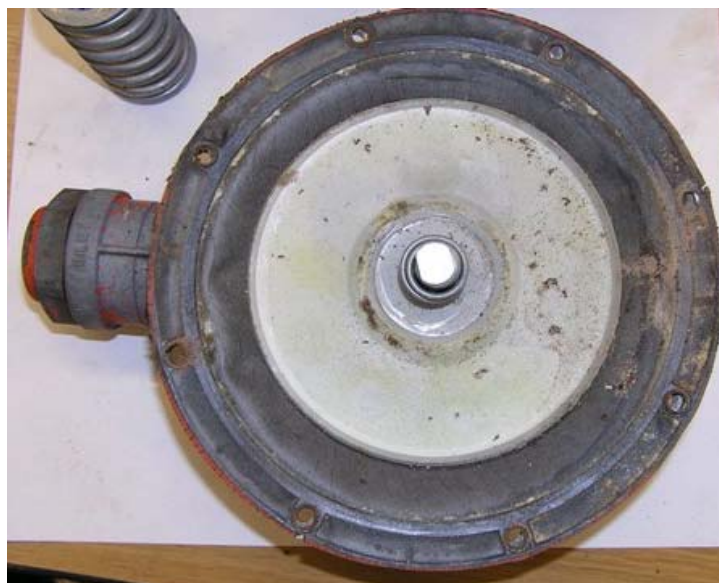
Figure 3: Diaphragm and Diaphragm Plate of Regulator #361
