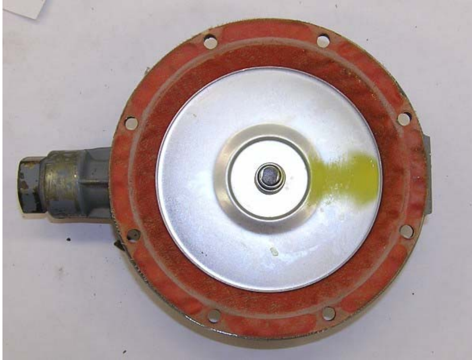
Figure 3: Diaphragm and Plate of Regulator #383
