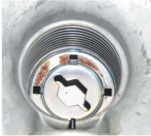
Figure 4: Bottom of Adjustment Spring Plate (Regulator #13)
