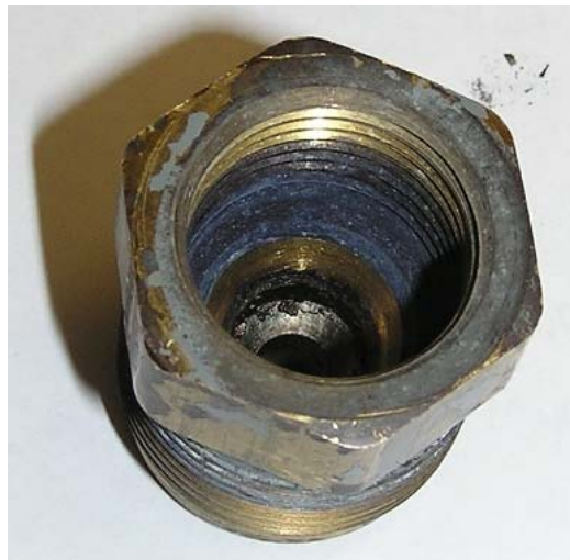
Figure 9: Inlet Side of Nozzle Orifice of Regulator #383
