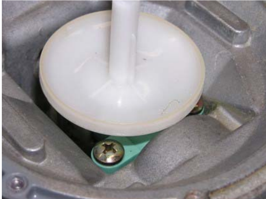
Figure 5: PRD Stem and Bottom of Second-Stage Body (Regulator #490)
