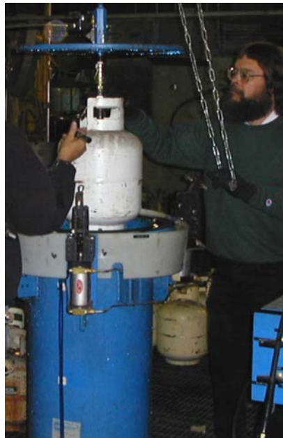
Figure A-4. Connection for attachment and internal pressurization of the propane tank before insertion in the water jacket.
