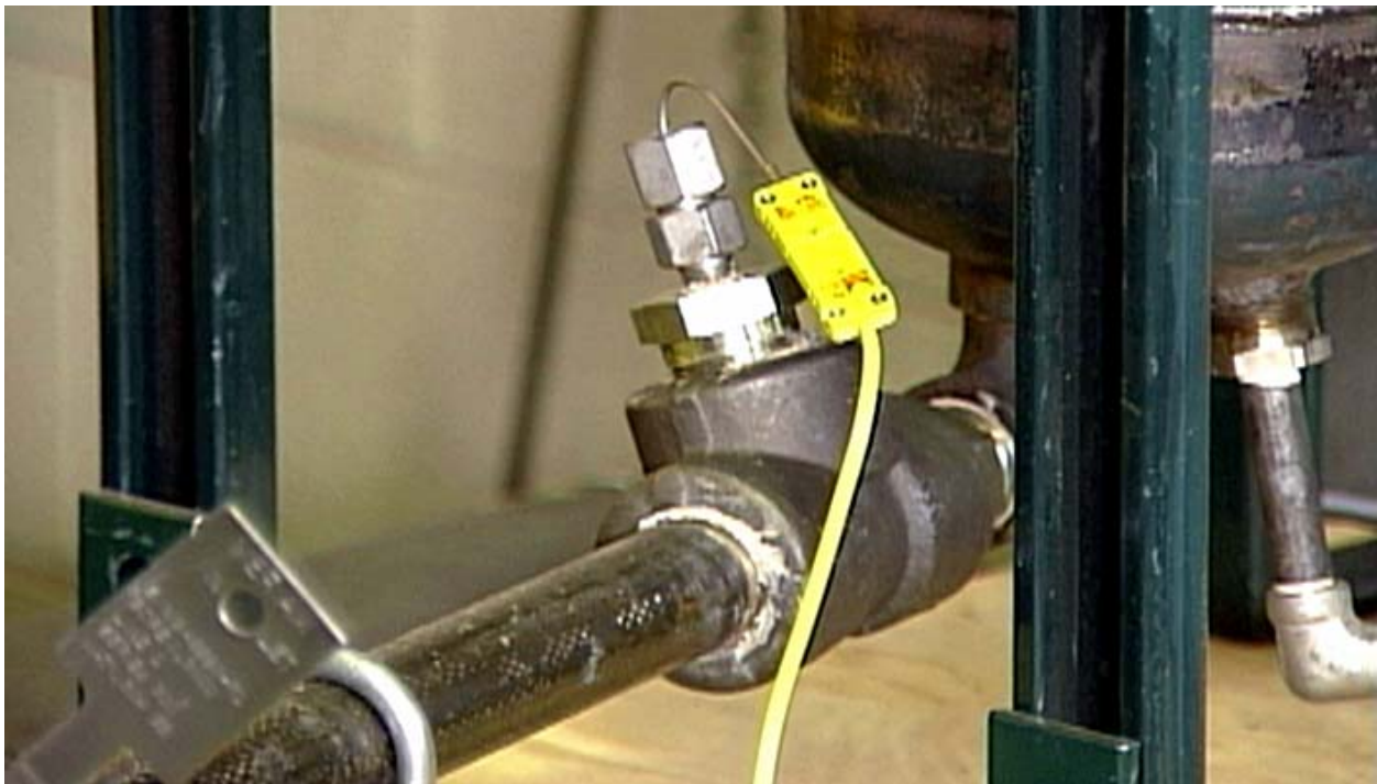
Figure A-12. Thermocouple used to measure temperature of applied air.
