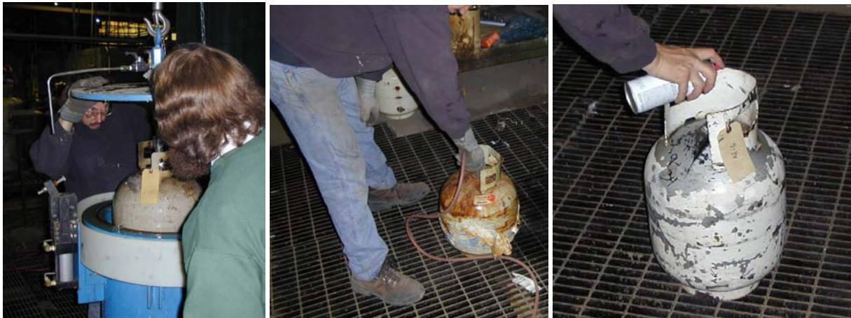
Figure A-8. Removal of the cylinder from the jacket, drying of the fracture surface with air and painting the fracture surfaces with clear acrylic paint to preserve their appearance.
