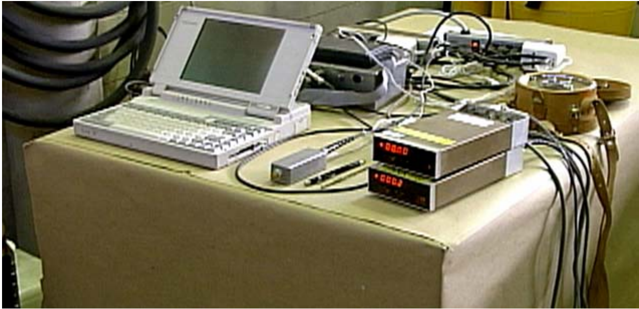
Figure A-16. Computer and data acquisition equipment used to monitor and record pressures and temperatures throughout testing.
