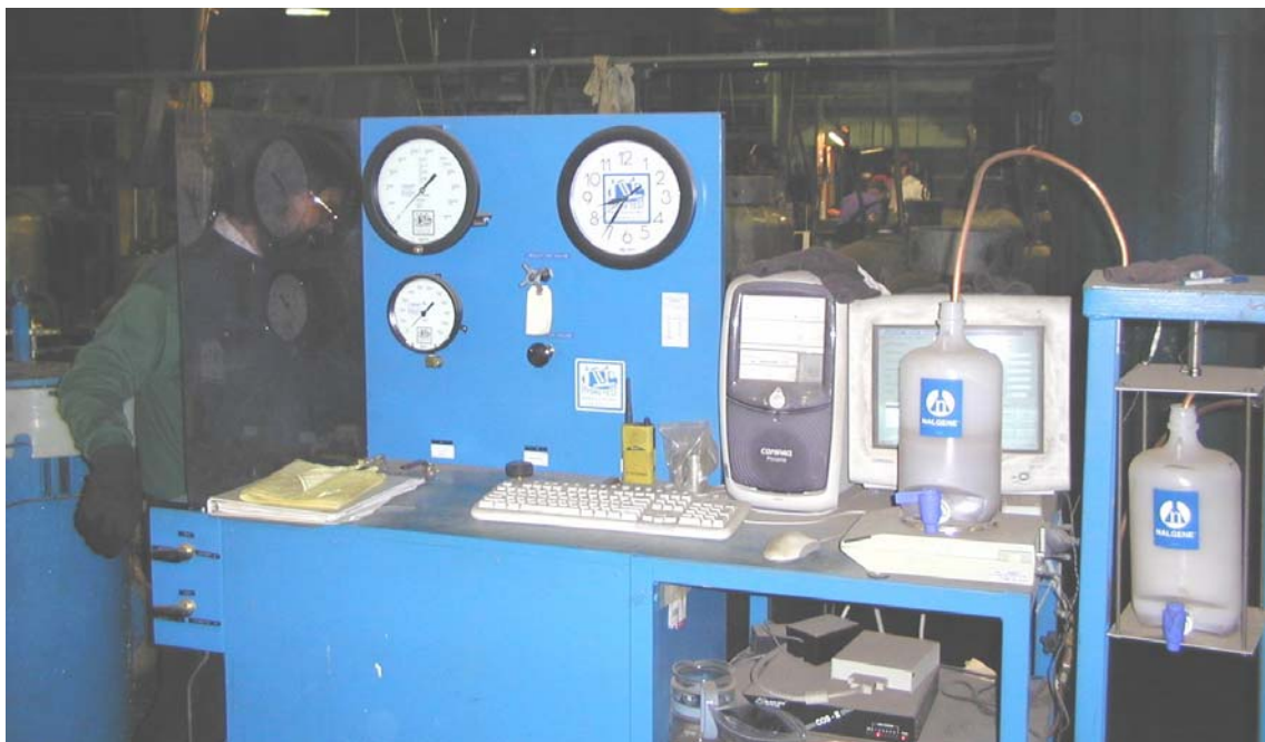
Figure A-6. Control panel and computer system for control and data acquisition of hydrostatic and burst tests.
