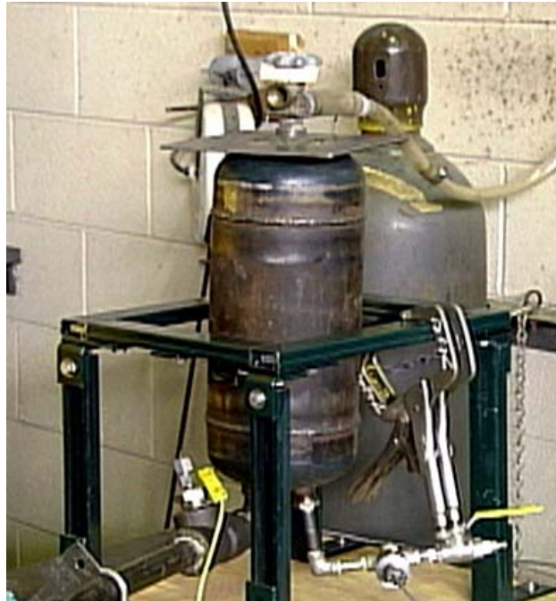
Figure A-13. Cylinder used to pressurized and test relief valves.
