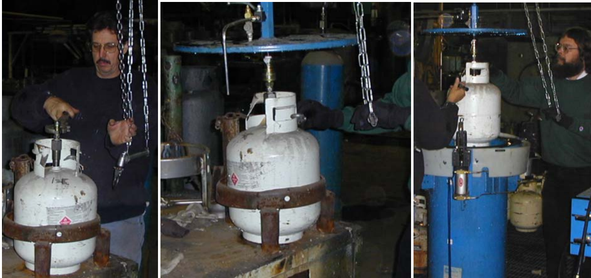
Figure A-7. Attachment of the filling connection and the lid to the cylinder, followed by insertion into the water-filled jacket.
