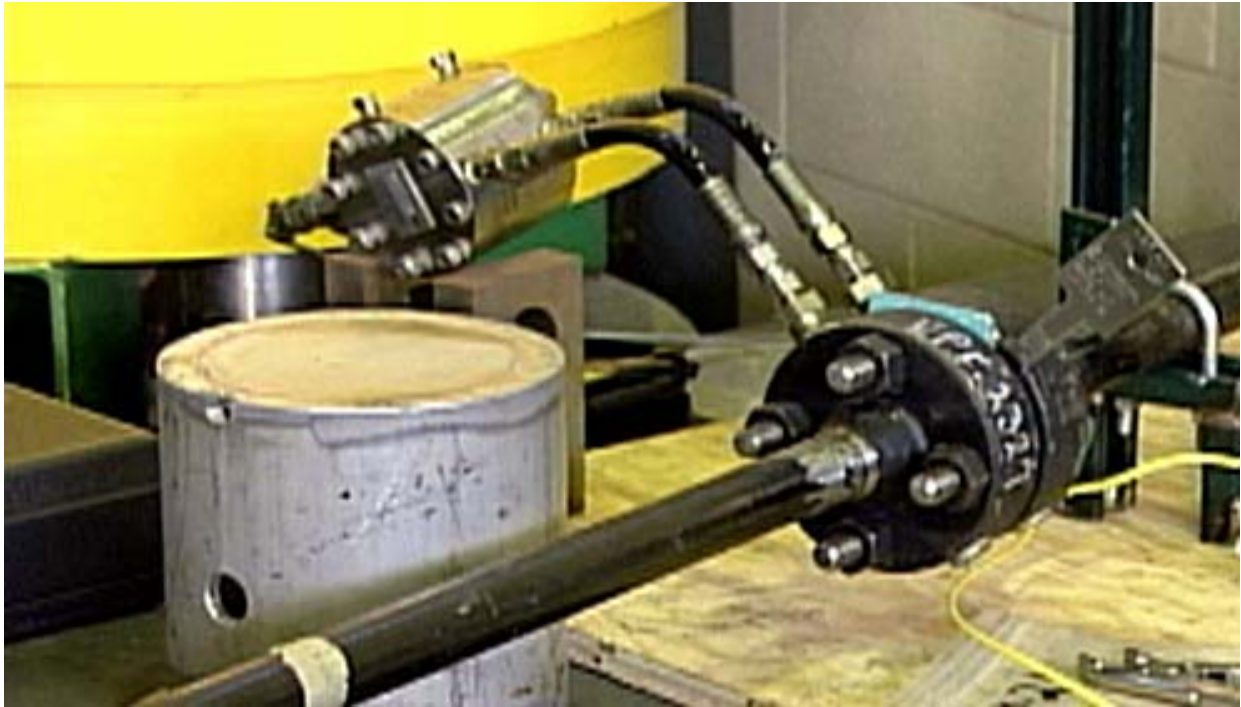
Figure A-11. Orifice and differential pressure sensor used to measure flow rate.
