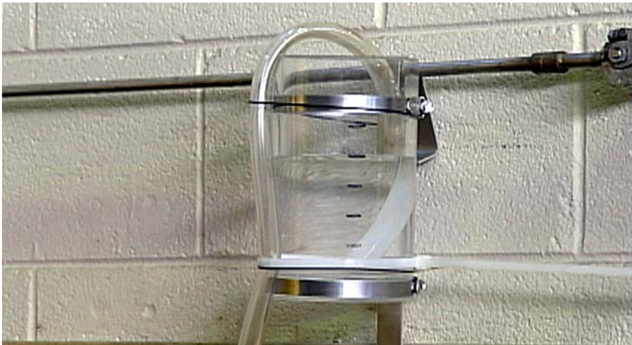
Figure A-15. Hose and reservoir used to monitor bubbling of air from relief valve.
