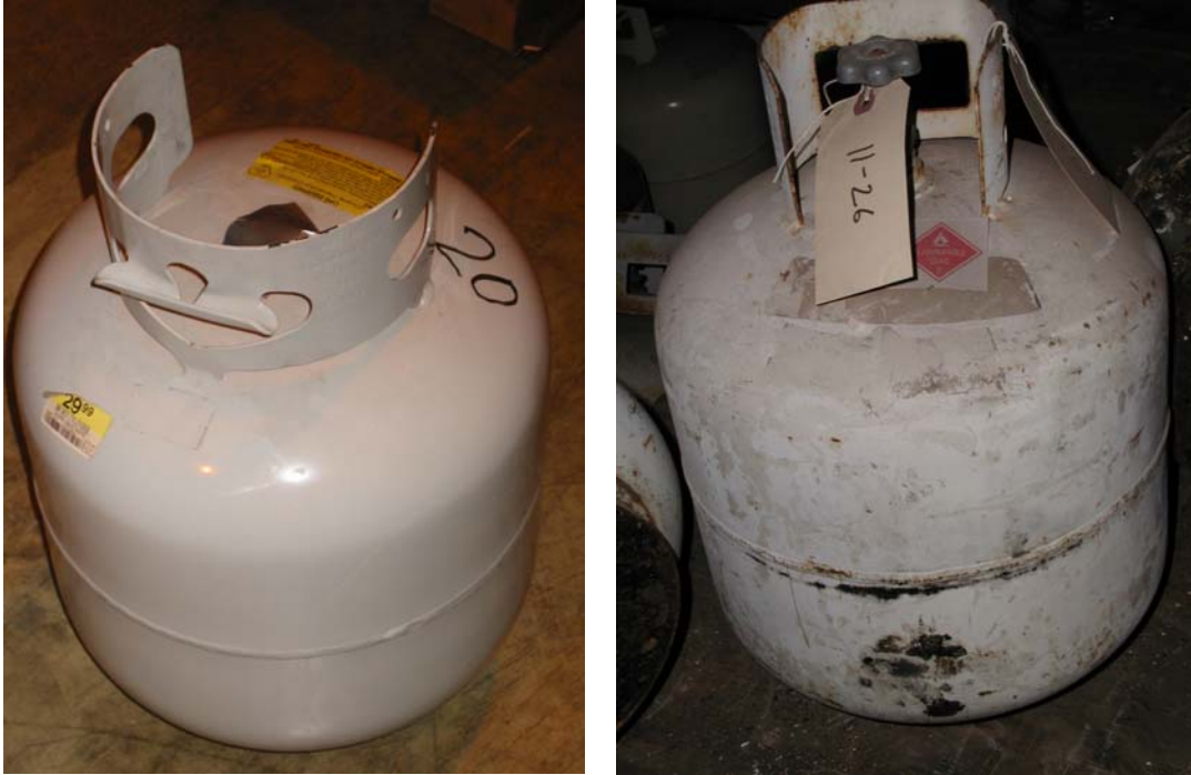
Figure 1. Examples of unused and used 20-pound LPG storage cylinders investigated in this program.
