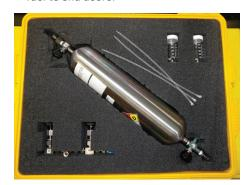
The fuel sampling kits include a 2.2-liter stainless steel cylinder (center) for collecting fuel, glass containers (top right) for collecting deposit samples, and a manifold (lower left).
